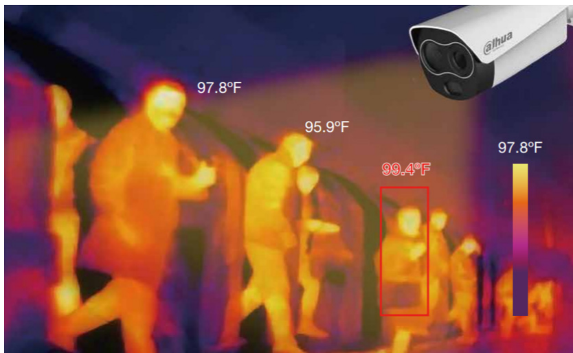
Dahua Technology's "Thermal Temperature Monitoring Solution" is capable of identifying individuals with an elevated temperature from a distance of three metres. Image: Dahua Technology handout, LewisSurveillance.com.
